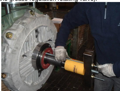
Removal of seals with puller
