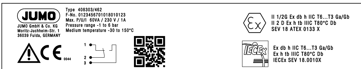
Fig. 3-3 Nameplate in Ex version flameproof enclosure, Ex d
