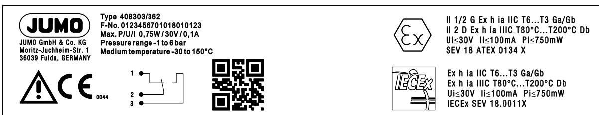
Fig. 3-2 Nameplate in version explosion protection intrinsically safe, Ex i
