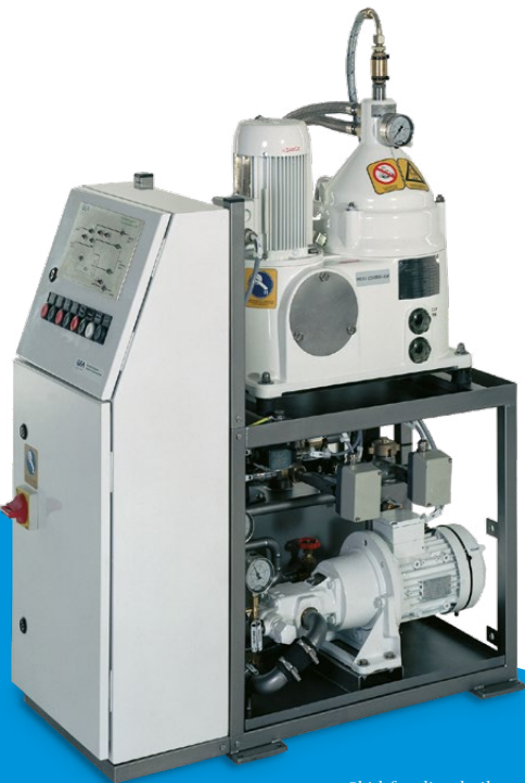
Skid for diesel oil treatment with a capacity up to 1,200 l/h
