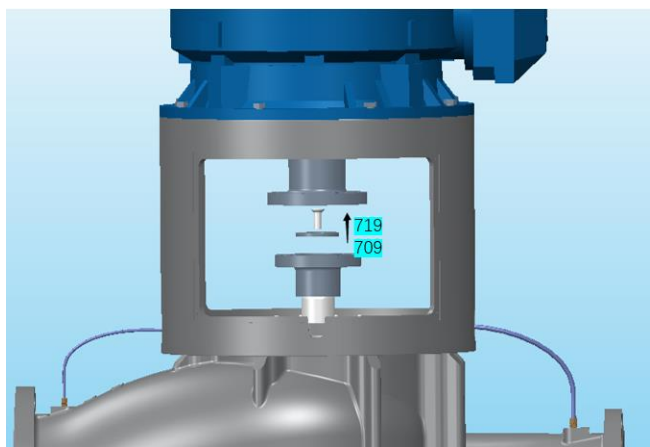
Remove screw (719) and plate (709)
